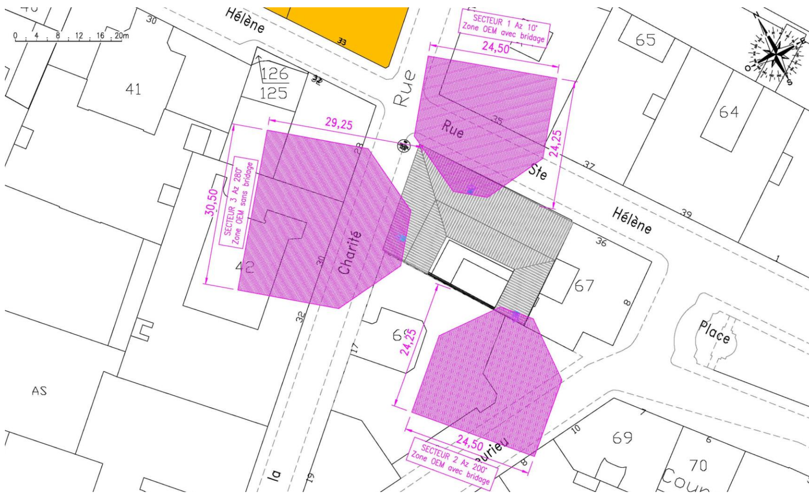
PERIMETRE DE SECURITE BOUYGUES TELECOM
